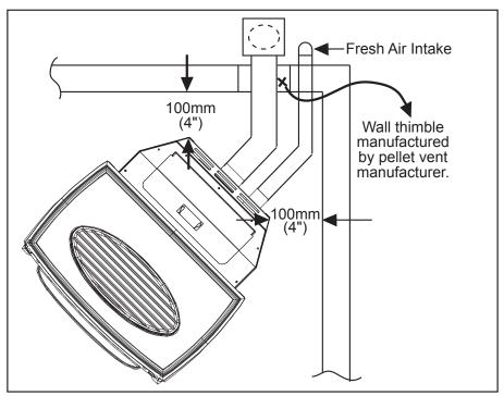
Figure 8: Corner Installation.
